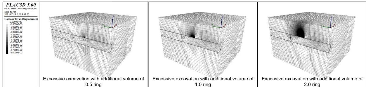
Fig. 3 Settlement diagram when excessive excavation occurred at wet ground
