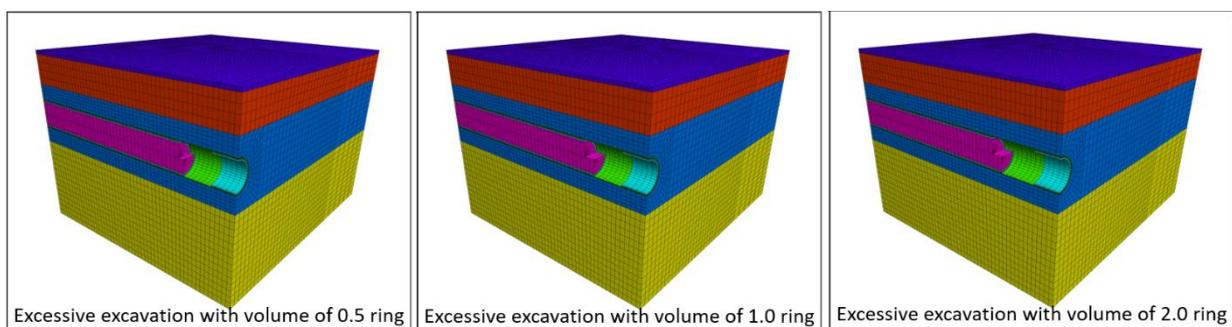
Fig. 1 Modelling of excessive excavation
